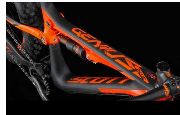
The full-suspension frames consist of super light and stiff HMX carbon main frames and Plus optimized alloy swingarms. The bridge of the Seat stay is built wider and stiffer than ever before. It is specifically formed and put further down to guarantee even more clearance. Our proprietary IDS-SL dropout system (Interchangeable Dropout System-Super Light) is ready for the 148x12mm Boost standard. The Genius 700 Plus frame is also compatible with 29" wheels.
