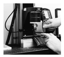
When designing a flat-resistant tire, puncture protection is paramount. Utilizing a proprietary, interwoven Polyamid matrix that is seamlessly bonded with the rubber compound, the Armadillo Elite vastly outperforms the previous Armadillo in the nail in tread test. Because the Polyamid casing is so densely woven it prevents punctures from outside debris, yet is also able to remain flexible enough for increased ride quality.
