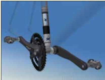
WORGL, Austria—Gruber's electric-assist, 200-watt motor is designed to fit within a 31.6-millimeter seat tube and drive a custom Hollowtech II-style bottom bracket axle through bevel gears. As long as the seat tube is straight and meets the bottom bracket shell close to the middle, the system will work. Since the system drives the crankset, it integrates seamlessly with a bike's drivetrain. The motor assist is turned on and off with a switch on the end of the handlebars. The en-
