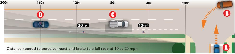
Perception & reaction time = 2.5 seconds. Braking distance based on median skill level.
