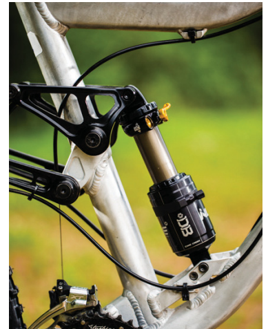
The DBinline shock fits a broader range of frames thanks to the elimination of the piggyback reservoir on previous Cane Creek dampers. The shock is the product of more than four years of development.
