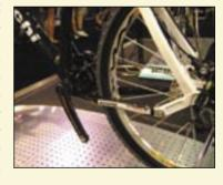
from how the carbon flex plate is laid up in manufacturing. Flipping the chainstay upside down does not alter the 80 millimeters of travel. The Camos, with a mix of XT and XTR, sells for \$6,100. It's handmade in Italy by a carbon supplier to Ferrari.
