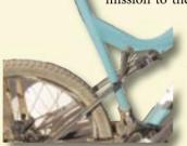
grated seatpost," said Chris Conroy, Yeti's general manager. The company figures it saved 80 grams over a traditional seatpost while boosting torsional stiffness close to 50 percent over the '07 ASR Carbon. In addition to providing different seatpost mounts that allow adjustability, Conroy said riders can cut the seat mast off, add a clamp and run a traditional 27.2 seatpost.
