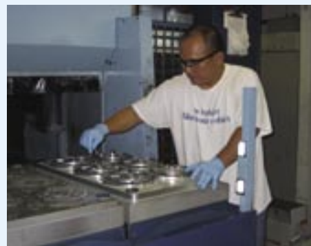
Edward Malunhao, one of the night-shift workers, loads Team Chainrings onto one of the CNC milling machines.
