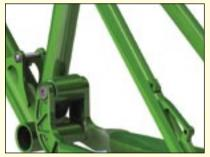
position can be optimized for pedaling while braking efficiency is optimized by the floating dropout—pivot-position compromise is no longer needed. The result is a bike with performance characteristics that will outshine the best single-pivot bikes in a package that can be as strong, light, cost effective or costly as needed. Weagle is pitching the Split Pivot to original equipment manufacturers.
